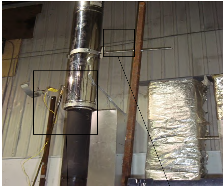
Gas analysis and temperature probe
