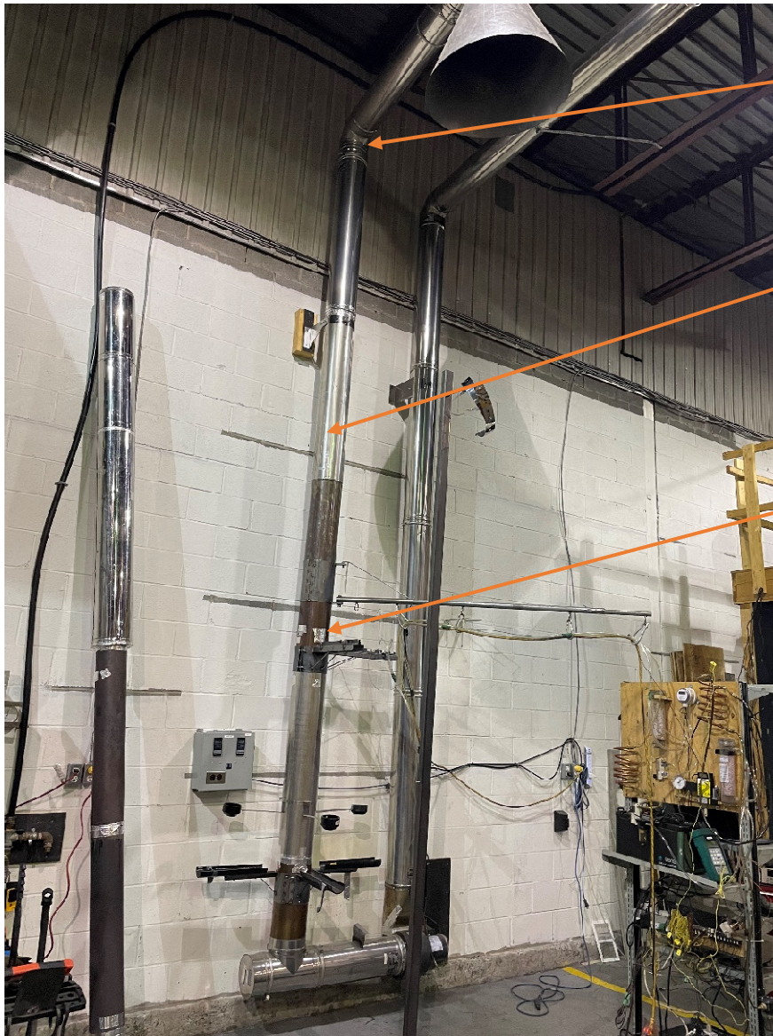
Total length between hood and sampling port: 23 feet.
