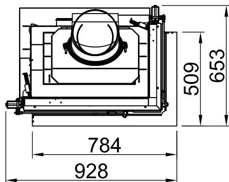
Front elevation view also shows a width dimension of 928.
